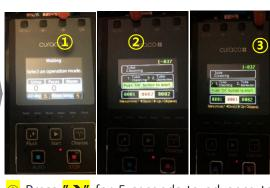
① Press "→" for 5 seconds to advance to function "1-037 Tube Cleaning"
