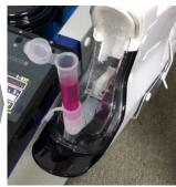
Open the silicon cap at the bottom and insert the Disinfectant Tube into the round hole on the plastic
